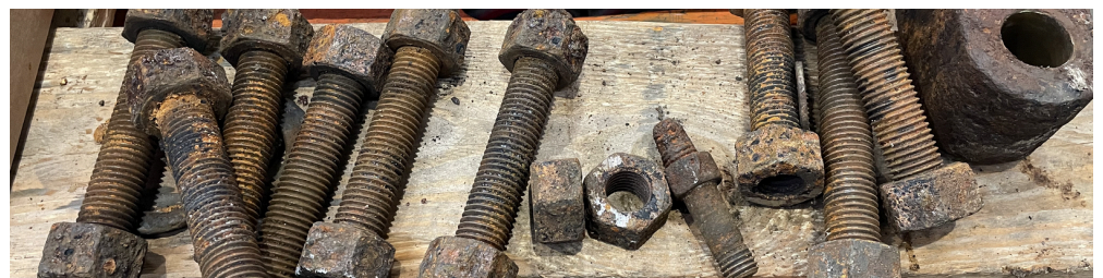
The Cover Fasteners were Badly Corroded
