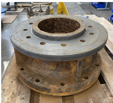
The Core Casting was in Reasonable Condition
