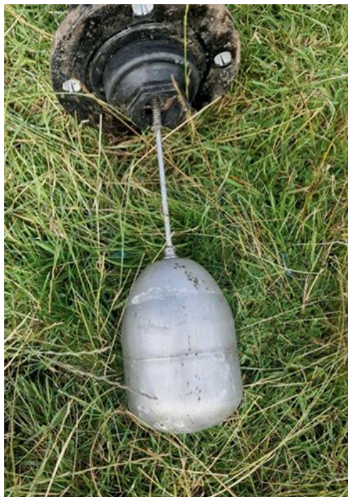
Air Valve float after service
