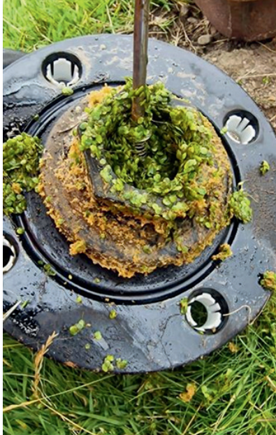
Seating mechanism packed with grease
