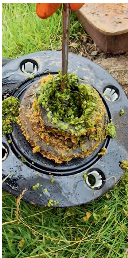
Seating mechanism packed with grease
