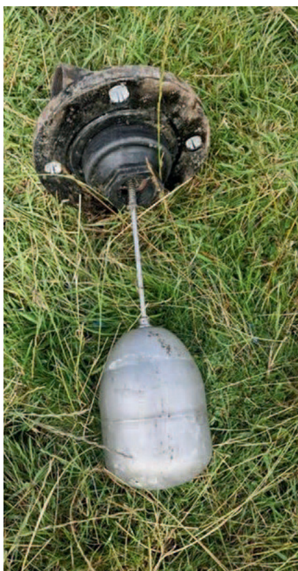
Air valve float after service
