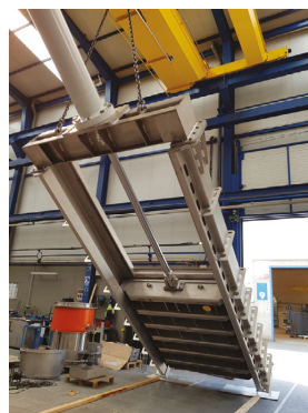
Primary Gate & Frame at Fat Inspection
