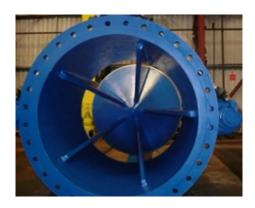
It is also imperative that the valve is correctly sized. Sizing calculations are based on the required discharge through the valve at the corresponding available pressure head. If not done correctly, this could lead to major issues with the valve itself, the overall discharge system, and the surrounding boundary surfaces. If undersized, the valve would not be able to achieve the specified emergency drawdown.
