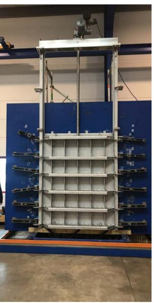
Penstock undergoing factory leakage and function testing.
