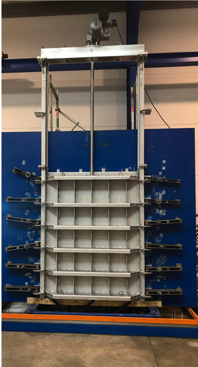
Penstock undergoing factory leakage and function testing.
