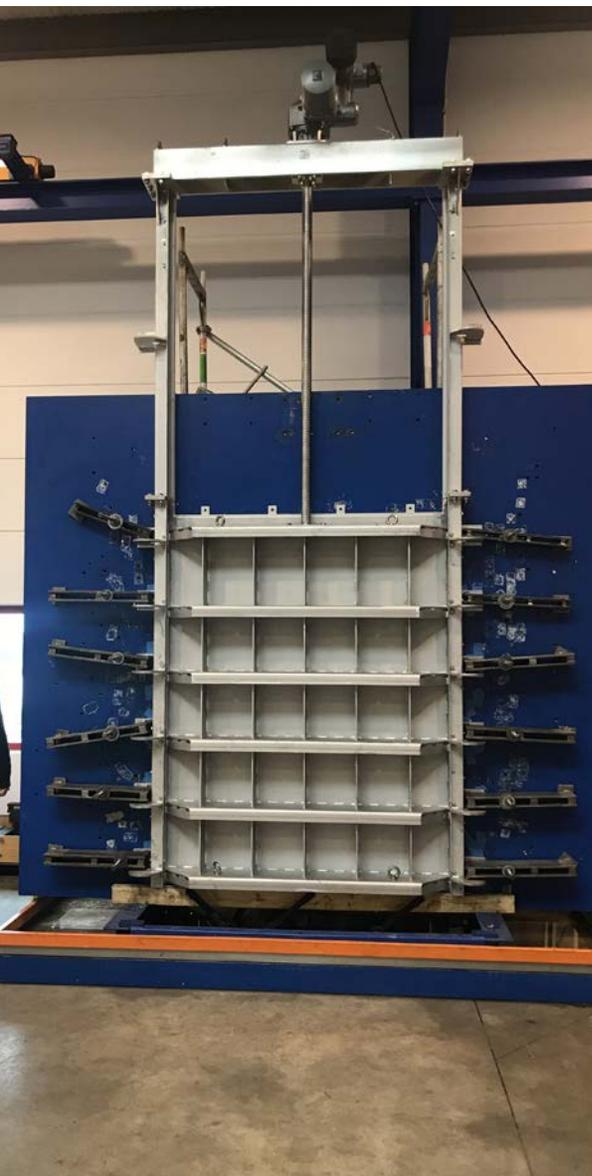
Penstock undergoing factory leakage and function testing.
